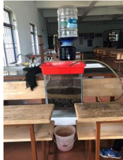
Fig.1. Filtration process in vermifiltration model
